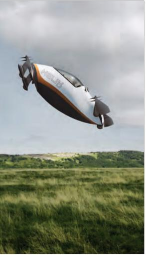
In hover mode, all propellers point upwards.
